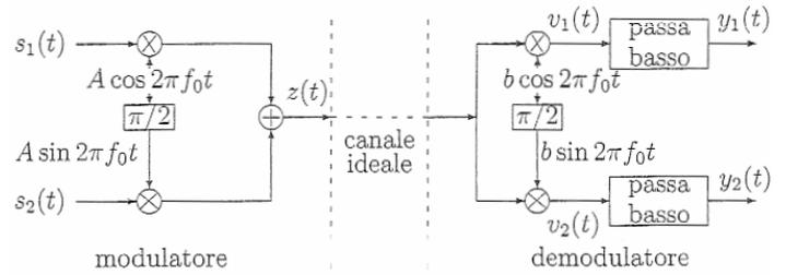
$y_1(t) = \frac{Ab}{2} s_1(t)$   $y_2(t) = \frac{Ab}{2} s_2(t)$   $\eta_{s_{QAM}} = 1$
